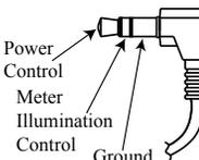
on McIntosh Power Amplifiers. A 3.5mm stereo mini phone plug is used for connection to the Power Control, Trigger and Passthru Outputs.
