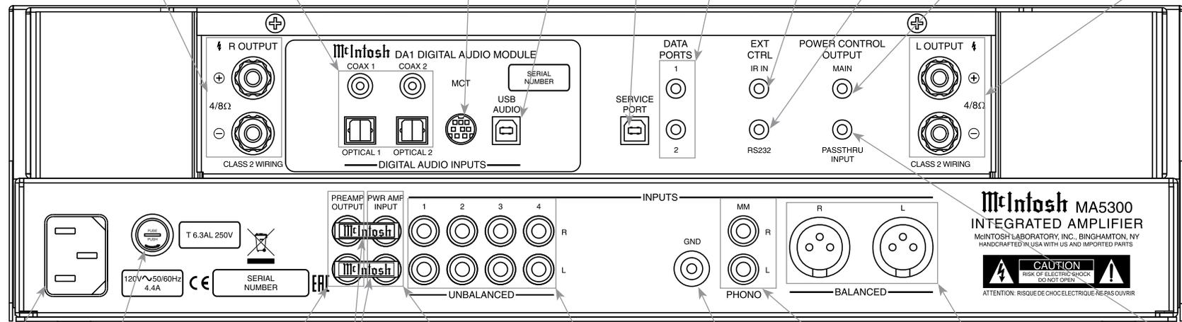
Main Fuse holder, refer to information on the back panel of your MA5300 to determine the correct fuse size and rating
